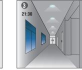
After 21:30, when all the people sensor automatically no back and stay at dim level 10% with the expiration of hold-time 10min.
