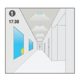
the Dusk/Dawn At sunset Photocell feature starts to work. When the amhient lux level is below the preset lux value. sensor will automatically turn on the light to dim level 10%, even if there is no movement around.
