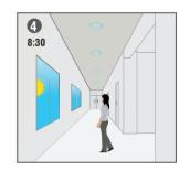
In the early morning, the Dusk/Dawn Photocell feature starts to work again. When the ambient lux level becomes above the preset lux value, sensor will automatically switch off the light. Thanks to the **Daylight Prior to Motion** feature, even if there is constant movement around during the process, the sensor will switch off the light accurately without any trouble.
