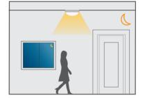
The light switches on automatically when natural light is below daylight threshold and presence is detected.
