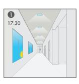
At sunset, the <u>Duck/Dawn</u> <u>Photocell</u> feature starts to work. When the ambient lux level is below the preset lux value, sensor will automatically turn on the light to dim level 10%, even if there is no movement around.
