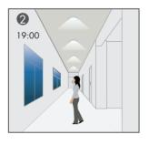
Between 17:30 to 19:00, when there is no movement around, light will stay at dim level 10% until people come at 19:00 and trigger the lights to 100% brightness level.
