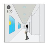
In the early morning, the <u>Dusk/Dawn Photocell</u> feature starts to work again. When the ambient lux level becomes above the preset lux value, sensor will automatically switch off the light. Thanks to the <u>Daylight Prior to Motion</u> feature, even if there is constant movement around during the process, the sensor will switch off the light accurately without any trouble.
