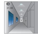
After 21:30, when all the people left, the sensor will automatically go back and stay at dim level 10% with the expiration of hold-time 10min.
