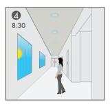
In the early morning, the <u>Dusk/Dawn</u> Photocell feature starts to work again. When the ambient lux level becomes above the preset lux value, sensor will automatically switch off the light. Thanks to the <u>Daylight Prior to Motion</u> feature, even if there is constant movement around during the process, the sensor will switch off the light accurately without any trouble.
