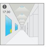
At sunset, the <u>Dusk/Dawn</u> Pho<u>tocell</u> feature starts to work. When the ambient lux level is below the preset lux value, sensor will automatically turn on the light to dim level 10%, even if there is no movement around.
