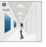
Between 17:30 to 19:00, when there is no movement around, light will stay at dim level 10% until people come at 19:00 and trigger the lights to 100% brightness level.
